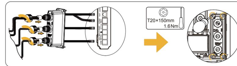
4.11. Refer to the battery quick installation guide to mount the cable covers. Refer to the inverter quick installation guide of chapter 8 to mount all covers.
