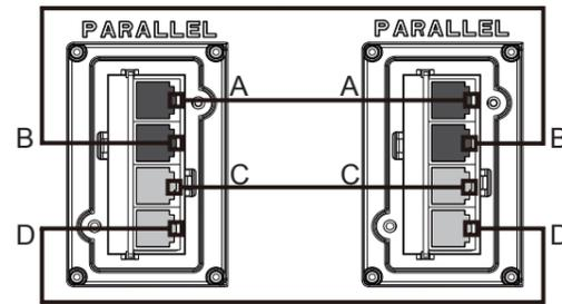
e. When securing the COM cover over the communication ports, tighten the cover in place and then lightly push the PARA COM cables into the cover as you tighten the strain relief nut onto PARA COM cables. This will ensure PARA COM cables are well-seated in the RJ45 sockets.
