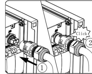
Electrical connection between grid connectors of the inverters and grid combiner cabinet have finished.
