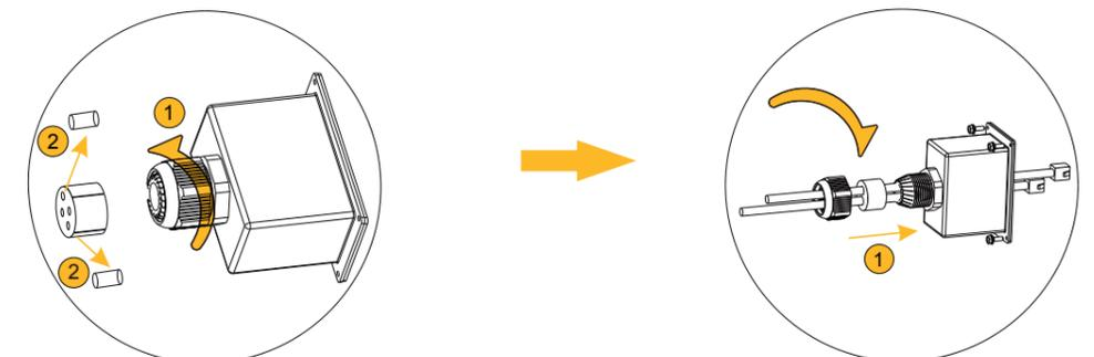
d. Wire the communication connection of inverters operation in parallel
