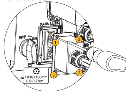
3.10. Install the WiFi modules or LAN cables connection to the inverters. Configure the network and put the inverters online.
